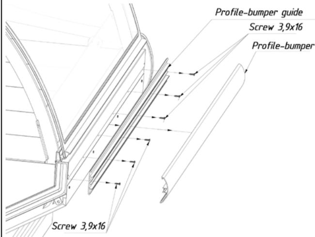
3.8.2. Unscrew 3,9x16 screws and remove front panel. Peel off the paper tape; leave a butyl sealing cord on the display body - it is designed to seal the connection of the displays.
