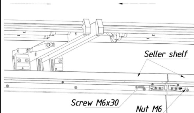
3.7.9. Secure the fan panel to the divider. Connect the storage chambers and the caps of the refrigerated display cases.
