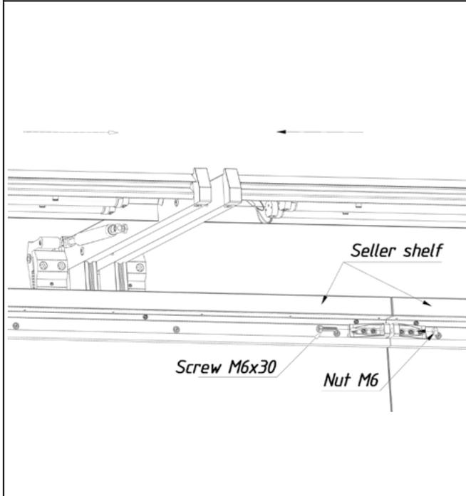
3.9.8. Secure the fan panel to the divider. Connect the storage chambers and the caps of the refrigerated display cases.
