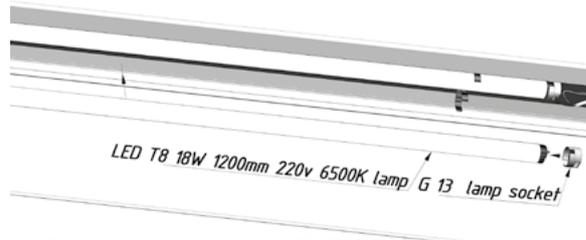
3.15.3. Connect the terminals to the G13 socket of the new lamp.
