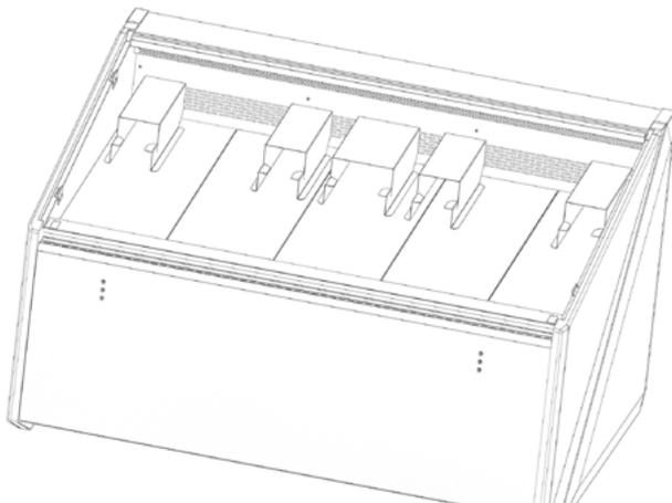
3.13.2. Place the bottom part of the stepped layout on the horizontal stainless steel layout by inserting the back of the segment of a stepped layout in the corresponding fixing groove of a rack of a stepped layout.
