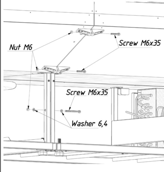
3.8.7. Install the displays so that the mounting holes are on the same axis.
