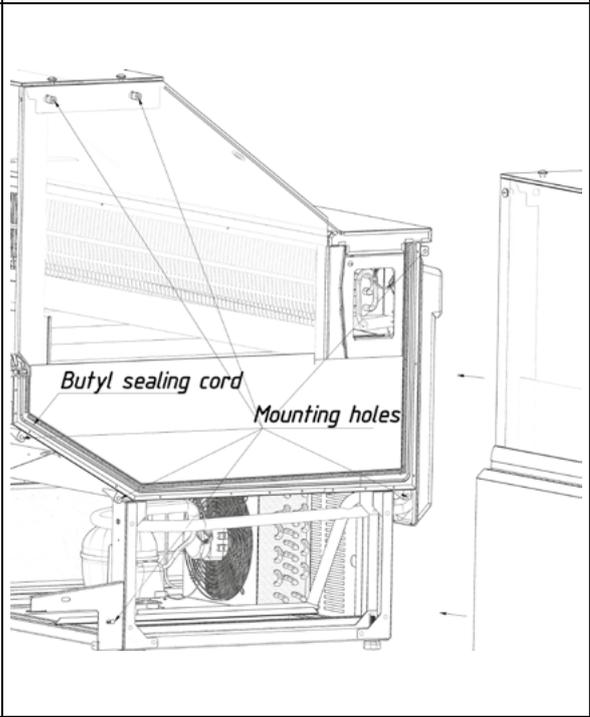
3.6.5. Connect the displays together using the fasteners included in the set. Connect the horizontal uprights with M6x45 screws. Close the holes with a decorative cap.
