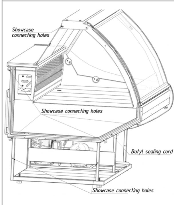
3.8.4. Connect the models together using the fasteners included in the set.
