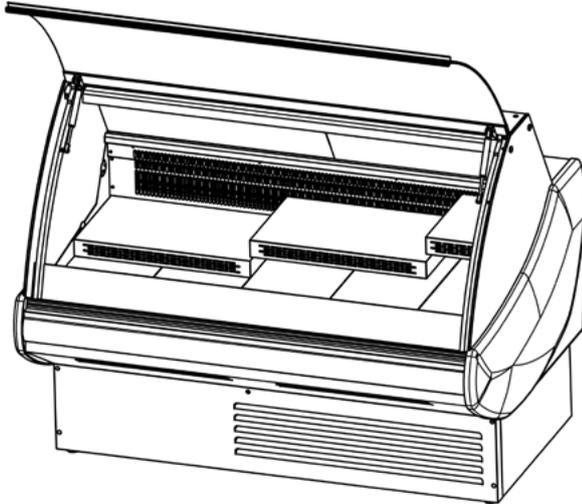
3.14.2. Ensure close location of the stepped layout to the evaporator grill.
