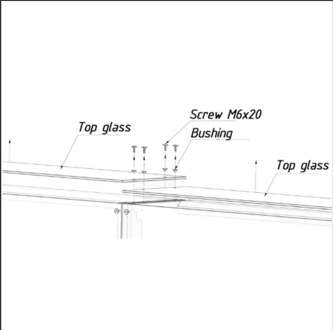
A technical line drawing showing the fastening mechanism for the top glass. The glass panel is held in place by two screws. Labels indicate "Top glass", "Screw M6x20", and "Bushing". The screws are shown passing through the glass and into a metal frame. The drawing is a perspective view from the side. |
