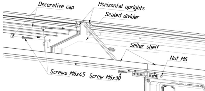
3.6.6. Use the level to ensure the horizontal positioning of the display. Mount the decorative panel in the panel-mounting hook and fix the bottom with fasteners.
