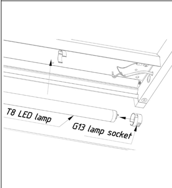
7.2.4. Connect the terminals to the G 13 socket of the new lamp.
