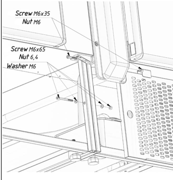
3.8.6. Connect the models together using the fasteners included in the set.
