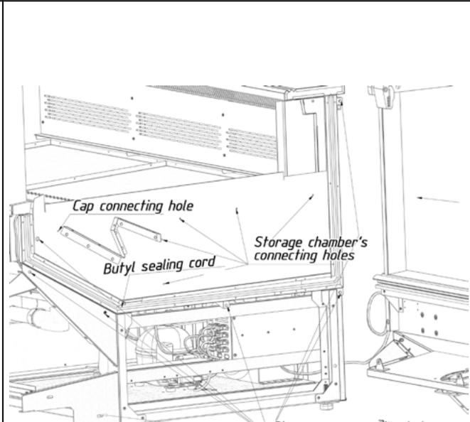
3.9.7. Connect the models together using the fasteners included in the set.
