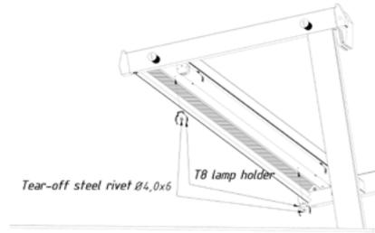
3.15.2. Connect the terminals to the G13 socket of the new lamp and install the new lamp.
