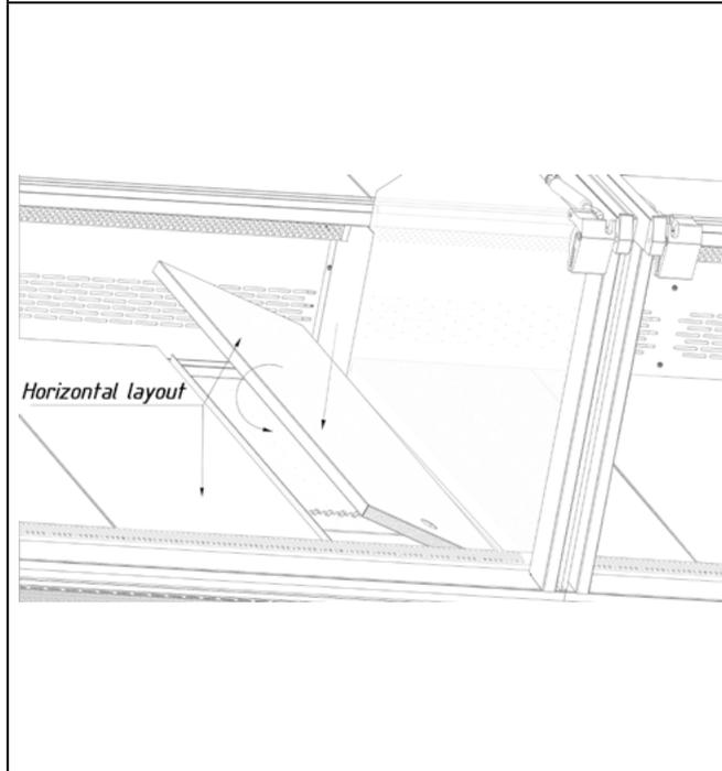
3.7.14. Install a sealed divider in the gap between the display racks and fix them with screws. Close the hole with a decorative cap. Install the upper and front glass.
