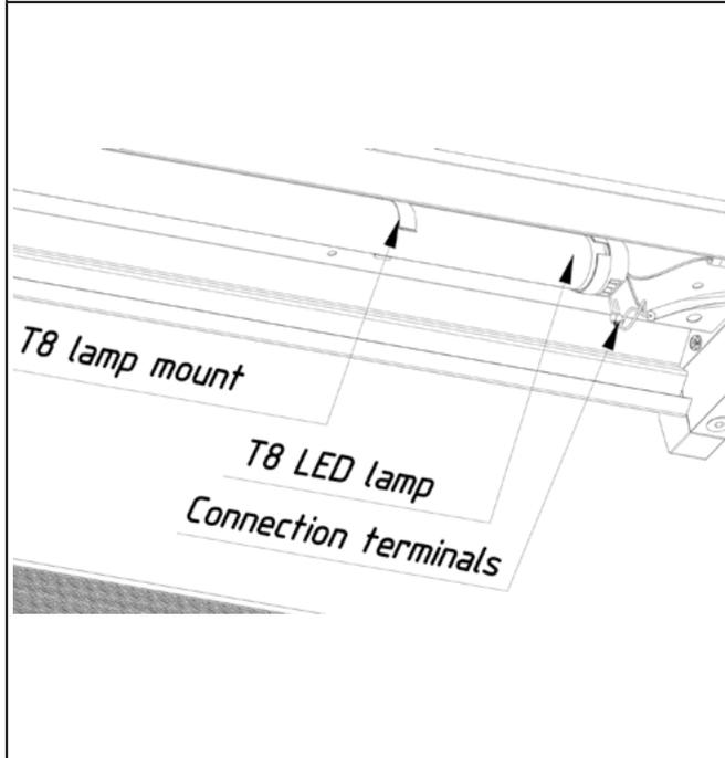
7.2.2. Remove the LED T8 lamp from the holder and disconnect the G13 socket.
