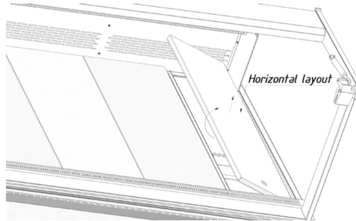
3.7.4. Unscrew the 3.9x16 screws and remove the beveled edge profile.
