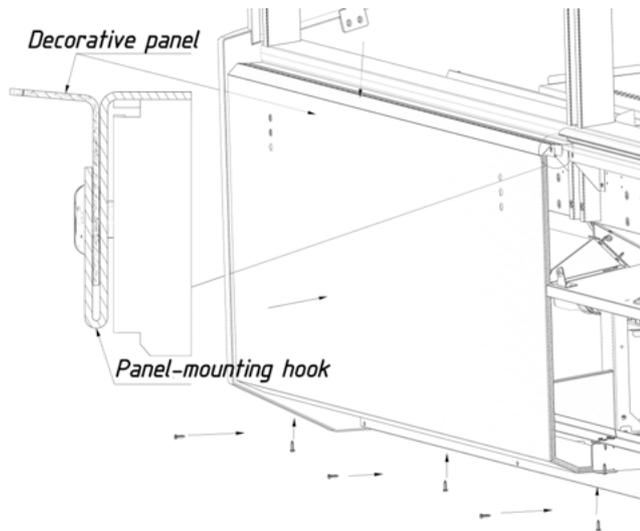
3.9.10. Install the beveled edge profile and fix with the 3.9x16 screws.
