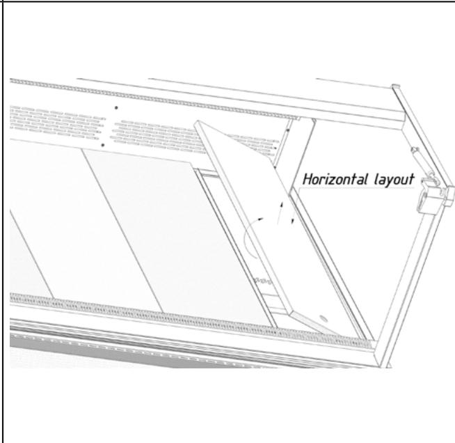
3.9.3. Unscrew the 3.9x16 screws and remove the beveled edge profile.
