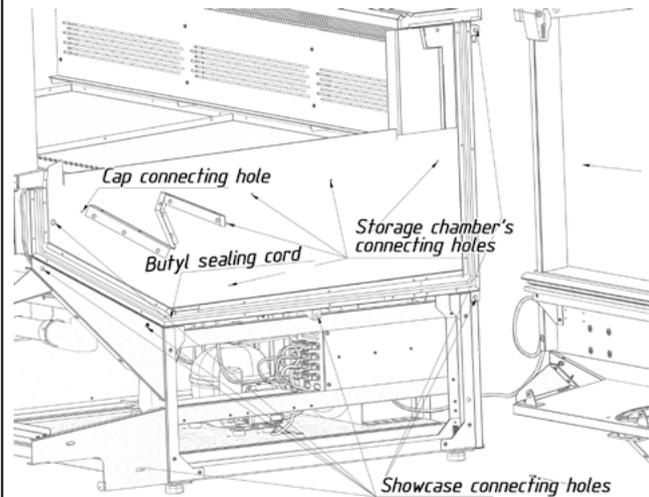
3.7.8. Connect the models together using the fasteners included in the set.
