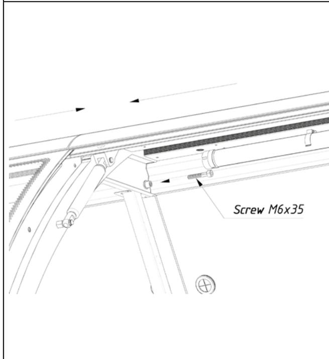
3.8.8. Use the level to ensure the horizontal positioning of the display. Install the profile-bumper and its guide on models assembled in line.
